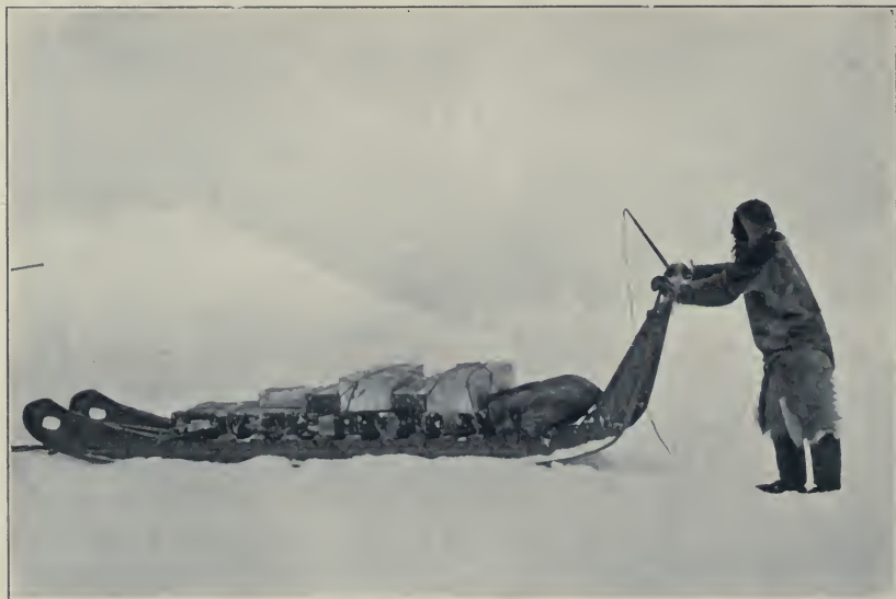
“PEARY” TYPE OF SLEDGE 12½ ft. Long, 2 ft. Wide, 7 in. High; With Steel Shoes 2 in. Wide
